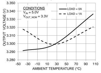
**Output Voltage vs. Temperature**
