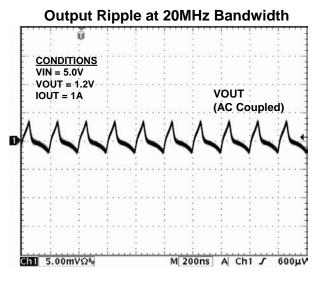
**Output Ripple at 20MHz Bandwidth**
