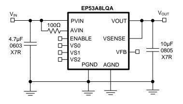
Figure 7. EP53A8LQA VID Application Circuit
