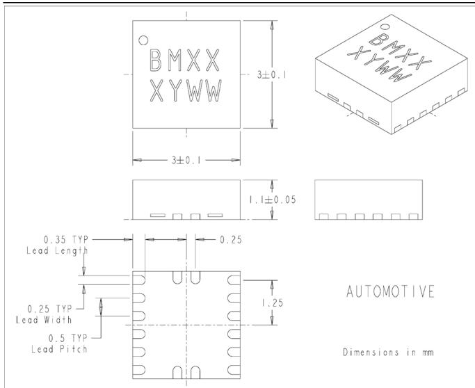
Figure 13. EP53A8HQA Package Dimensions (Bottom View)
