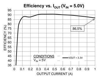
Figure 9. Efficiency vs. Output Current For  $V_{IN} = 5V$ ,  $V_{OUT} = 3.3V$  at 1A,  $\eta \approx 86.5\%$  $\eta = P_{OUT} / P_{IN} = 86.5\% = 0.865$  $P_{IN} = P_{OUT} / \eta$   $\mathsf{P}_{\mathsf{IN}} \approx 3.3\mathsf{W} \ / \ 0.865 \approx 3.815\mathsf{W}$
