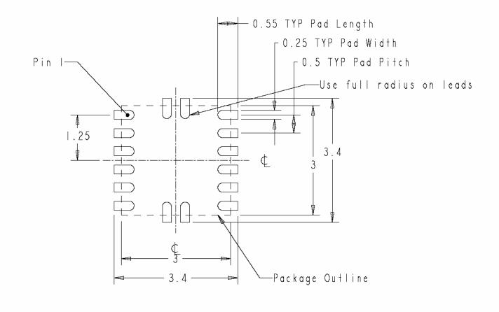
Figure 11. EP53A8xQA PCB Footprint (Top View)
