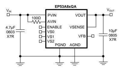
Figure 1. Simplified Applications Circuit
