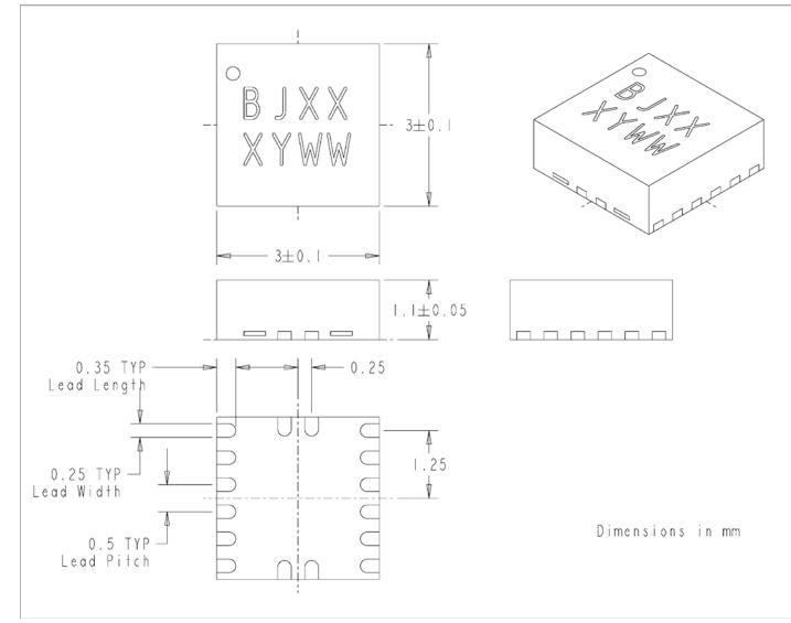
Figure 12. EP53A8LQA Package Dimensions (Bottom View)
