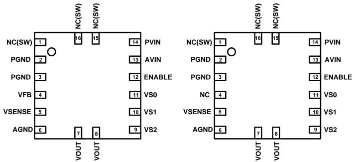
Figure 3. EP53A8LQA Pin Out Diagram (Top View)
