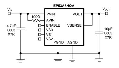
Figure 6. EP53A8HQA VID Application Circuit
