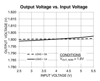
**Output Voltage vs. Input Voltage**
